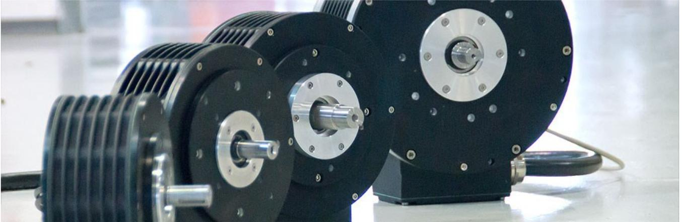
The PMSM is a brushless permanent magnet motor based on axial flux technology. The motor type is commonly referred to as “pancake motor” because of its flat design. Compared to a traditional induction motor the weight is lower and the efficiency is higher which means you can run your system longer and with less heating of the motor. The motor type also opens up for new applications where you cannot fit a larger motor.
