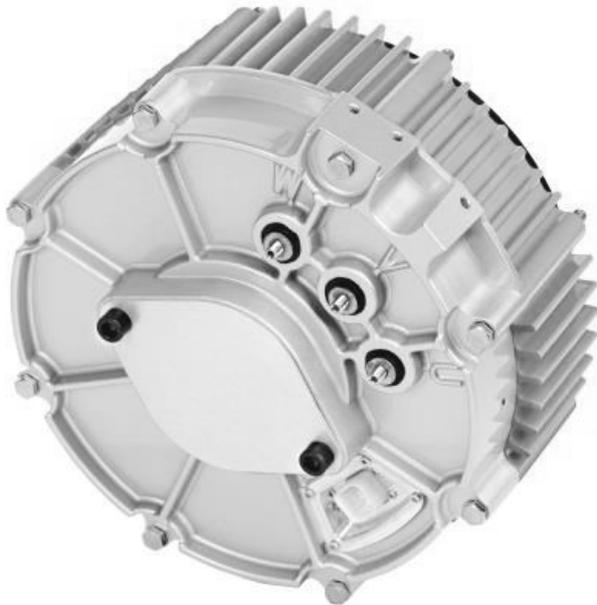
The GSM is a family of permanent magnet synchronous AC Generators with continuous **power levels from 14kW to 24kW** developed primarily for use in battery hybrid applications with nominal battery voltages **between 24V and 80V**. Other than the configurations listed in this datasheet the GSM can also be customized for other speed, power and voltage levels.
