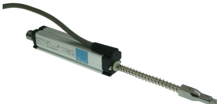
The KPY series is an absolute linear position sensor with a thru-rod design and return spring. The design has double rod support ensuring a greater strength and stability in a compact housing. KPY is a potentiometric sensor with high accuracy and wide temperature span.
